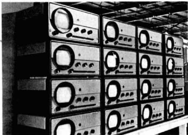
Early Hallicrafters television receivers are a collector's item now. This model had a push-button tuner that included TV channel 1, now the Amateur 6-meter band.
