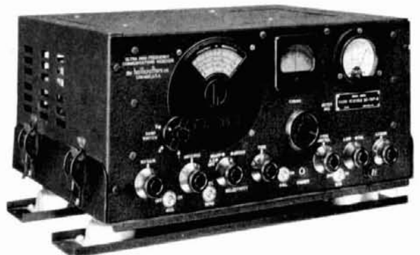
Large numbers of the Hallicrafters S-36 (BC-787B) receiver were sold during wartime. Tuning range was from 27 MHz to 140 MHz, which included vhf communications ranges of Allied, German, and Japanese ground and air forces. Receiver worked on both a-m and fm.
