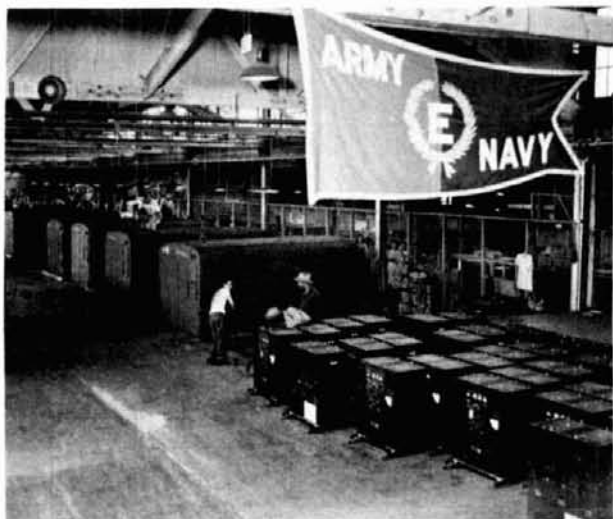
Hallicrafters won five Army-Navy E awards during World War II for excellence in production. This photo shows BC-610 transmitters in final inspection before they were mounted in the communications vans in the background.
