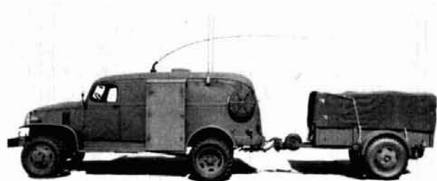
Always on the go! The SCR-299 communications truck was used to negotiate the surrender of Rommel, the "Desert Fox," in north Africa. The SCR-299 was present at the D-day invasion of Europe and accompanied General McArthur during his historic conquest of Leyte Island in the Philippines. Gasoline-powered generator is in trailer. Truck was supplied with three whip antennas for transmitting and receiving while in motion.
